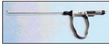
Figure 6a. Ellman Trigger-Flex Probe™ performing thermal discoplasty/annuloplasty. 4.0 MHz frequency shrinks the annulus and ablates inflammatory tissue effectively.
